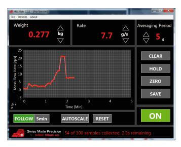
The user friendly software MSE Rate continuously samples the weight data of the load cells and calculates the actual gravimetric feed rate. MSE Rate is Windows™ based (XP, Win7/8) and runs on every PC with an USB 2.0 port. Its main features are:
